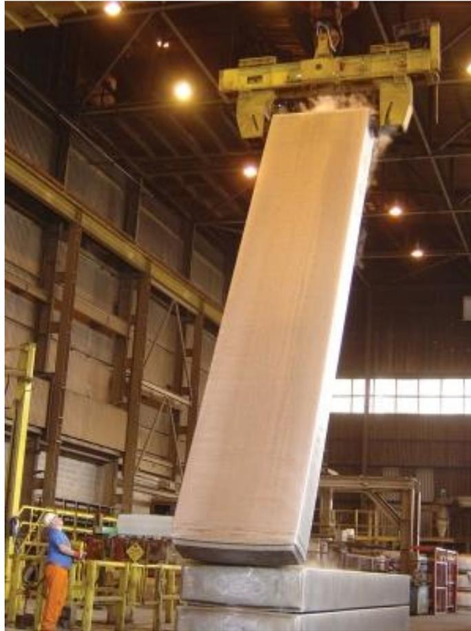
**7.) The finished ingots are lifted from the casting pit by an overhead crane**
